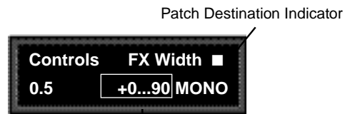
The FX Width value will be changing from 0 to 90 and back again.
