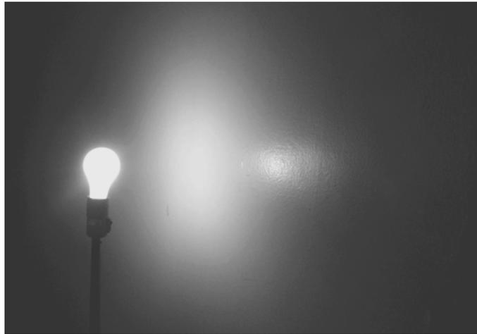
**Figure 2.1** Photograph of a wall surface which exhibits both specular and diffusive reflective properties. Note that there are two bright spots. The small area on the right is the specular reflection, the larger area in the centre is the diffuse component.
