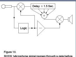
RODS: Microphone signal passes through a gate before going to a tapped delay line, and the output of the line goes through a similar gate. The logic opens the input gate and closes the output gate when the mike signal is steady or rising. It closes the input gate and opens the output gate when the level falls. This system does not increase lateral energy during continuous music.
