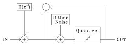
human psychoacoustic characteristics and reduce the apparent noise power levels. The effectiveness and resulting spectrum is highly dependent on the filter used. This application note presents several possibilities: a simple 1-stage delay:
